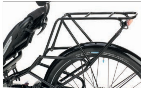
The stable rack for two panniers weighing up to 25 kg (55 lbs) has been optimized to withstand the high lateral forces to which trikes are subjected. The panniers are positioned down low with an optimum center of gravity, and close to the rider to the side of the rear wheel. 14 mm (0.6") tube. Ideally, you should accessorize it with the Top Load attachment, which is attached to the luggage carrier. This platform can carry up to a 10 kg (22 lbs) payload, particularly suitable for more substantial loads.
