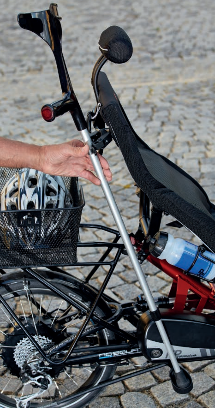
Walking aid mount: Easy insertion, safe transport and fast removal of walking aids. The practical fastener adjusts seamlessly to diameters from 20 to 31 mm (0.78 to 1.18 inches). HP VELOTECHNIK's stainless steel clip fixates the walking aid and releases it again with a non-fumbling one hand operation.
