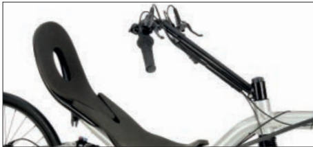
Alternatives for the cockpit: The Tiller steering handlebars combine a relaxed arm position with good aerodynamics. The hands lie loosely in front of the chest.
