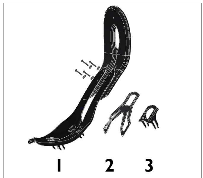
1 - BodyLink seat, 2 - mounting bracket, 3 - upper seat bracket
