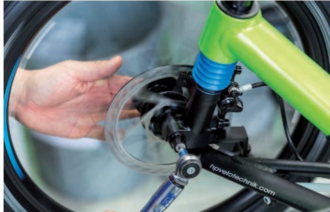
A front wheel finds its place on the forged high tensile strength wheel carrier of the Scorpion fs Enduro chassis. For this model blue bellows protect the strut.
