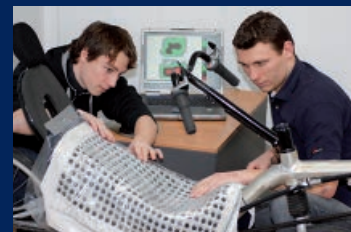
Computerized pressure distribution analysis on a BodyLink seat for the ideal shape.
