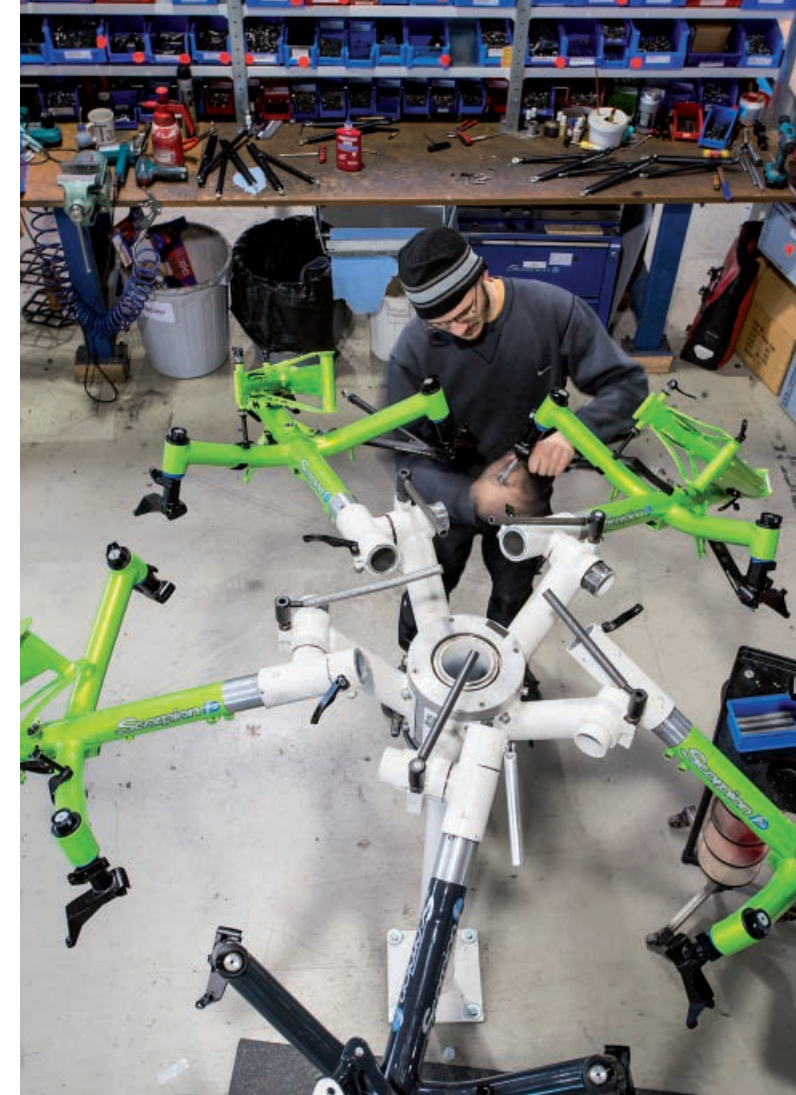
During pre-assembly the freshly powder coated enduro frames take a round trip on the carousel. Here the folding hinges and the suspension are assembled.
