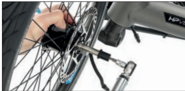
Easy to transport: HP VELOTECHNIK has developed open wheel mounts which allow the front wheels to be simply detached together with the brake disc by loosening just one bolt (HP Performance hubs standard on Scorpions).
