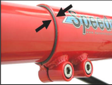
The plastic bush between front boom and main frame must be visible at all time.
