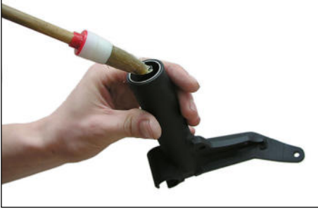
Applying grease to the bushings.
