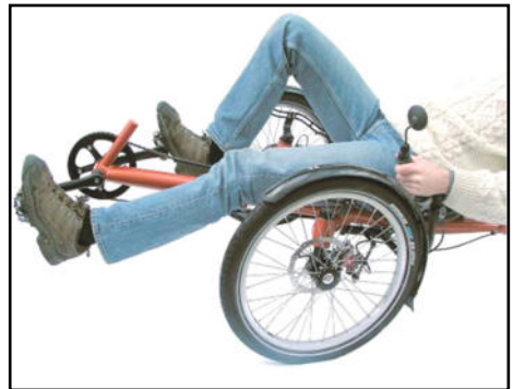
Adjust the front boom so that your knee will not be fully straightened when pedalling.
