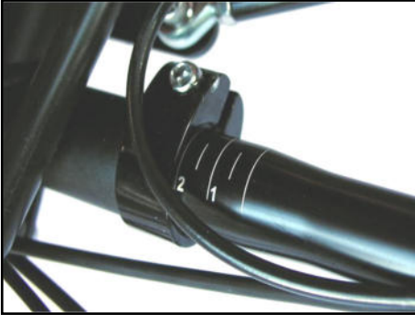
Handlebar width and angle are adjusted with the clamp at the stem under the main frame.
