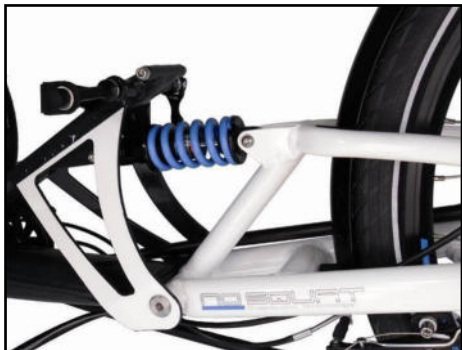
Steel spring suspension element with fixed damping rate.
