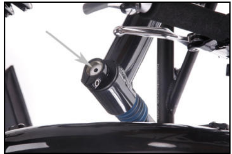
Hex head screw for adjustment of the pre-load for the spring inside the knuckle
