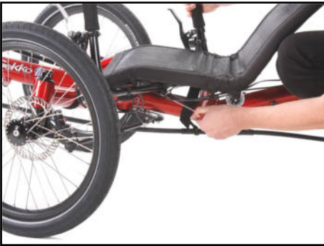
Handlebar width is adjusted at the stem clamp under the seat.
