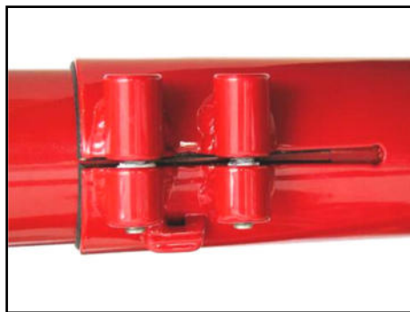
The rear end of the front boom must never be visible in the clamping slot.
