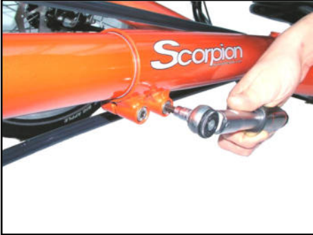
Loosen the bolts to adjust the front boom.
