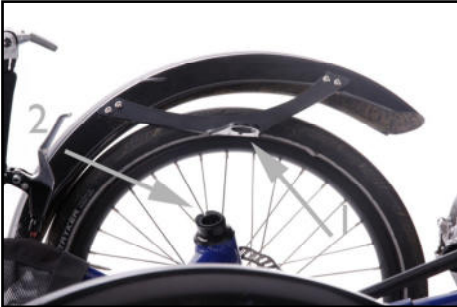
Mounting of front mudguards on Scorpion, Scorpion fx, Gekko fx 20, Gekko fx 26, and Gekko 26
