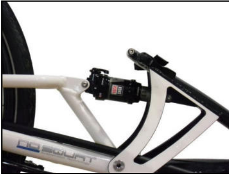
Air Shock ROCKSHOX Monarch damping is adjusted with the red knob at the rear end. Watch correct mounting direction depending on your model! (Lever facing upwards: Scorpion lfs 26 lfs 26 Enduro lfs 26 S-Pedelec lplus 20 lplus 26; downwards: Scorpion fx lfs 20)
