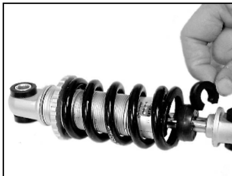
The suspension travel is adjusted by adding clips to the piston rod of the spring element.
