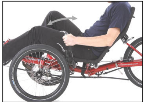
The handlebar angle is individually adjustable.
