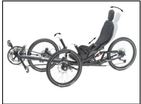
Seat adjustment on tricycles with BodyLink-seats
