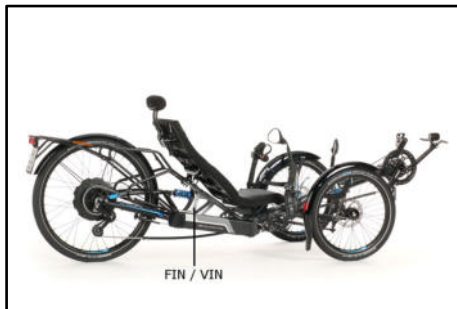
Position of the Vehicle Identification Number (short VIN; German: FIN)
