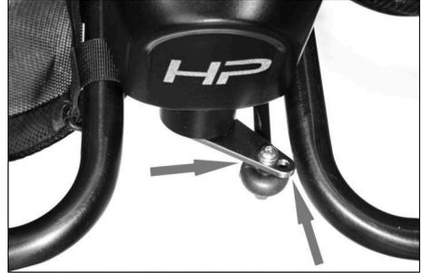
Fig. 13: For the attachment of the push rod and adjustment of the steering there are 2 threads on the steering lever to choose from.
