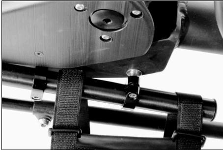
Fig. 10: The leg rest mesh is fixed behind the clamps
