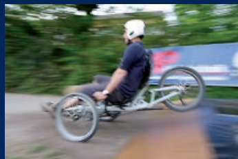
Overload testing during prototype test rides on the road and in more extreme situations
