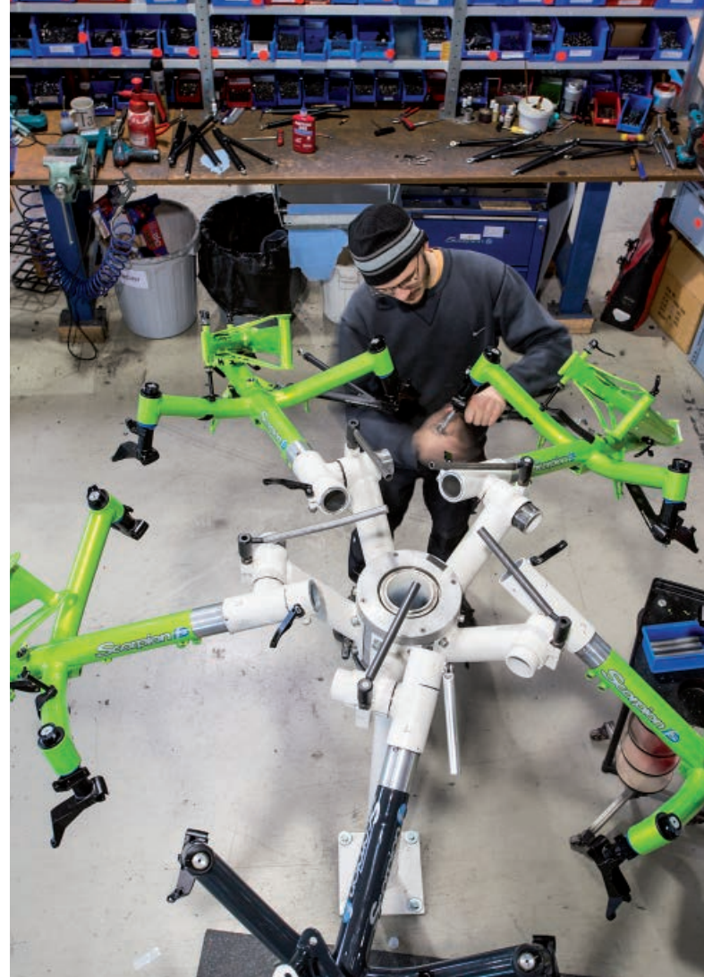
During pre-assembly the freshly powder coated enduro frames take a round trip on the carousel. Here the folding hinges and the suspension are assembled.
