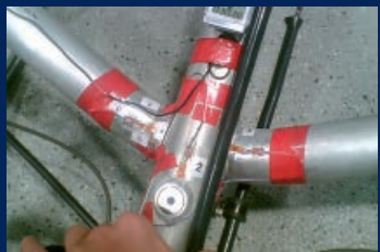
Measuring realtime material stresses for FEM analysis in the 3D CAD model.
