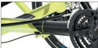
To adjust the frame to your leg length, you can slide the front boom into or out of the main frame after loosening the two clamping bolts under the main frame.
