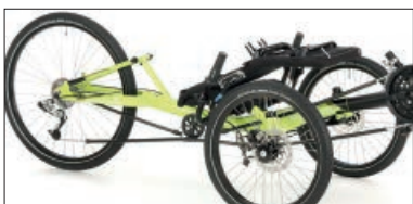
Convenient to transport: Although the Gekko 26 comes without a folding hinge for the main frame, you can still fold the seat forward to reduce the height when transporting the trike in the car.
