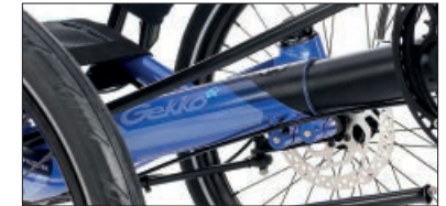
After loosening the two clamping bolts at the frame bottom, the frame is set to your leg length by sliding the front boom in or out from the main frame.
