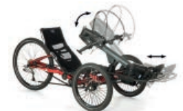
Hands-On-Cycle , the elegant hand drive for trikes. Outstanding: The worldwide unique concept with the completely enclosed chain guide has a turning circle just as small as the trike with foot drive.
