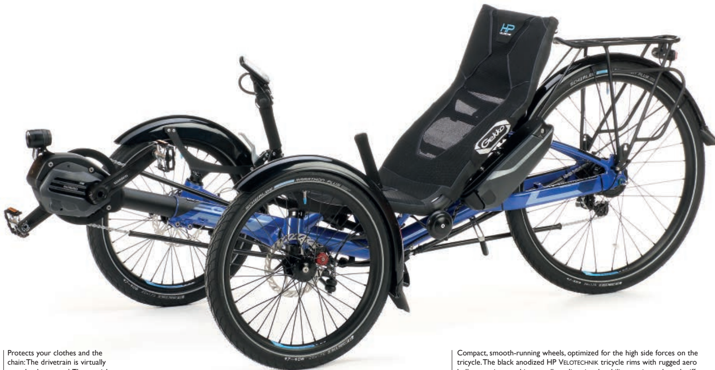
With the optional Quick frame adjustment, the length can be adjusted more quickly. The chain length modification is compensated by smooth pulleys. By sliding in the front boom during transport, your Gekko fx 26 is even more compact.
