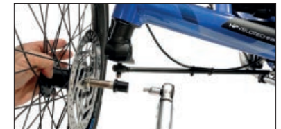
Practical during transport: HP VELOTECHNIK has developed unique open knuckles: With the HP Performance hubs the front wheels can be removed easily along with the brake discs by loosening a single screw. (Performance hubs are standard on Gekko fx 20, Gekko fx 26 and Gekko fxs models)
