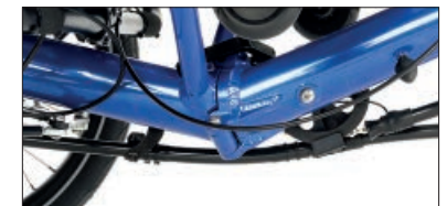
Double safety: The sturdy folding joint has a safety bolt that is unlocked against spring pressure after the quick release is disengaged. Stainless steel precision folding axis from HP VELOTECHNIK.
