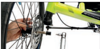
To reduce the size of your Gekko 26 even further, loosen the axle bolts of the HP Performance hubs with an Allen key and simply remove the front wheels together with the brake disc.
