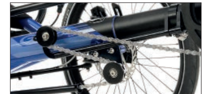
With the optional Quick frame adjustment, the length can be adjusted more quickly. The chain length modification is compensated by smooth pulleys. By sliding in the front boom during transport, your Gekko fx 26 is even more compact.
