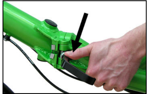
Open the quick release lever, then push the quick release down to unlock the security bolt of the folding hinge
