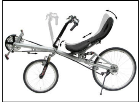
Adjustability of the BodyLink seat (here: Streetmachine Gte with tillerbar)
