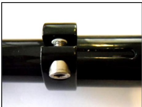
Clamping of the height adjustment for above seat steering. The end of the upper stem half must not be visible in the clamping slot.
