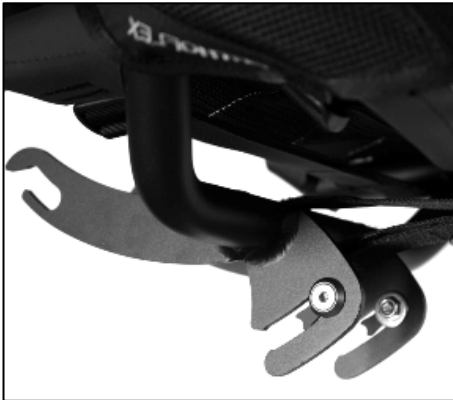
End stops mounted on a ErgoMesh Premium seat to ensure handlebar free movement on a Streetmachine Gte
