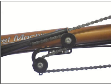
Routing of the chain over the idlers of the front boom quick adjust
