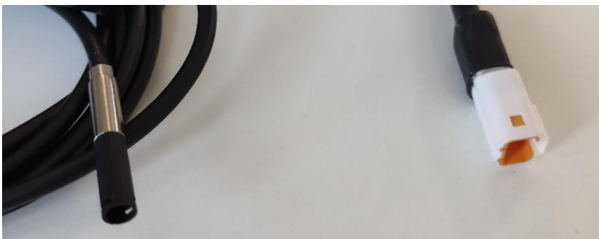
Figure 4: adapter cable with neodrive connector (left) and with JST connector (right).
