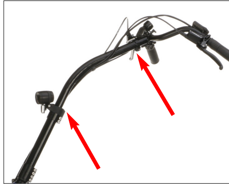
Minimum insertion depths of the stem parts: The clamping slot (middle part) resp. the hole (lower part) of the outer stem part must be completely covered by the inserted stem part.
