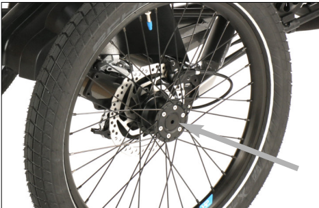
The central bolt needs to be opened.
