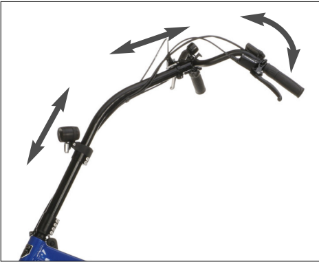
Adjustment options of the Delta tx stem
