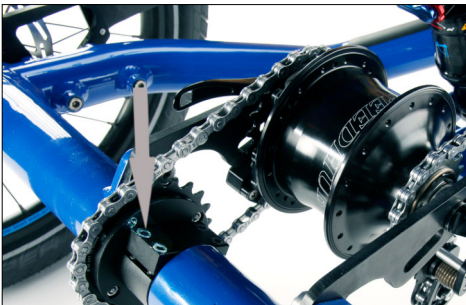
When dismantling the right rear wheel or mounting the left rear wheel: Use a chain whip to fix the axle mounted sprocket.
