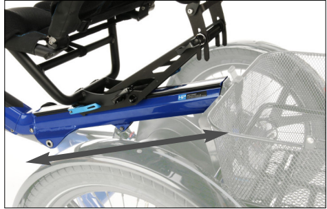
The seat adapter can be slid on the rear frame for adjustment
