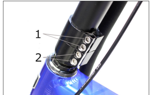
1 - Allen screws to secure the stem on the fork. 2 - Torx screws for the fork clamping
