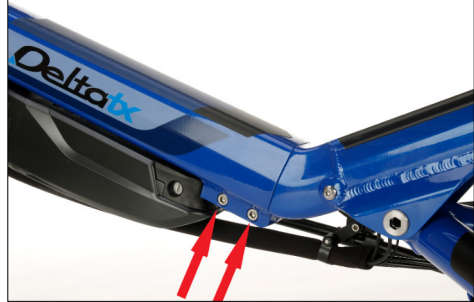
The M6 screws clamp the frame.
