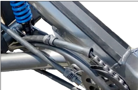
Slide the chain between the swingarm's tubes.
