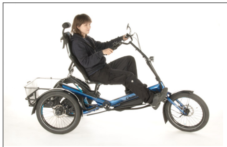
Short stem middle part, shortened by 20 mm (0.8"), rider height 1.61 m (5.3 ft)
