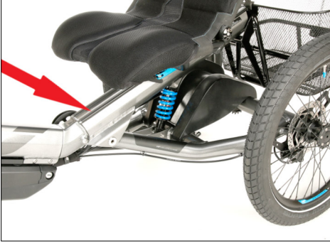
The frame number is placed on the left side of the frame at the beginning of the seat rail.
