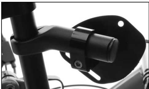
Attachment bolt M5x16mm of pivotal clamp
