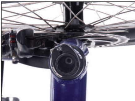
View into head set with star fangled nut inside
