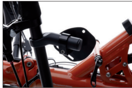
Attachment bolt M5 x 16 of pivotal clamp
