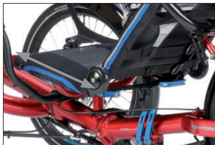
The seating length can be slid in or pulled out.
