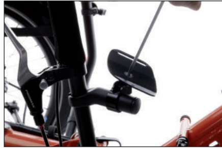
Adjustment of the handrest plate
