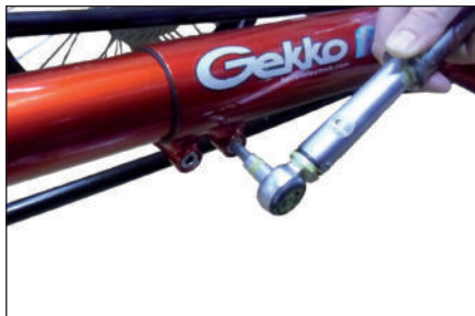
Loosening the bolts to adjust the front boom
