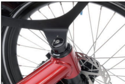
The holding sheet of the mudguard is fixed with the cap to the head set.
