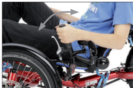
The handlebar angle is individually adjustable.
