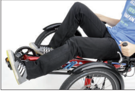
Adjust the front boom so that your knee will not be fully straightened when paddling.
