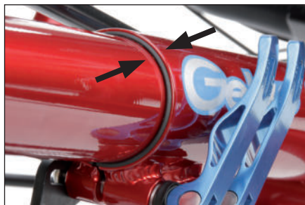
The plastic bush between front boom and main frame must be visible at all time.
