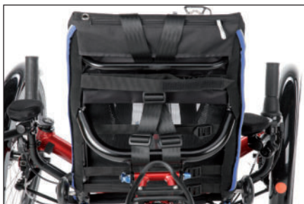
Positioning of the harness belt
