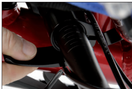
Handlebar stem clamp with quick release lever
