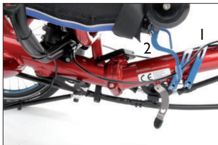
Rear frame with frame quick release levers (1) and seat quick release levers (2)
