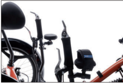
Handrest on both sides with one retaining strap
