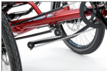
Routing of the chain over the idlers of the front boom quick adjust
