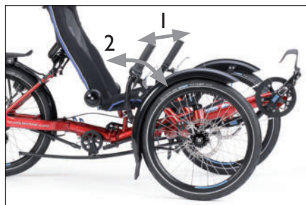
The handlebar allows adjustment in width (1) and angle (2)
