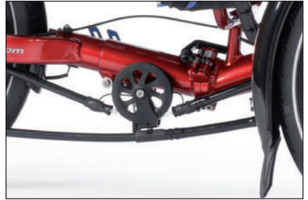
Chain roller and chain tubes on Gekko fxs
