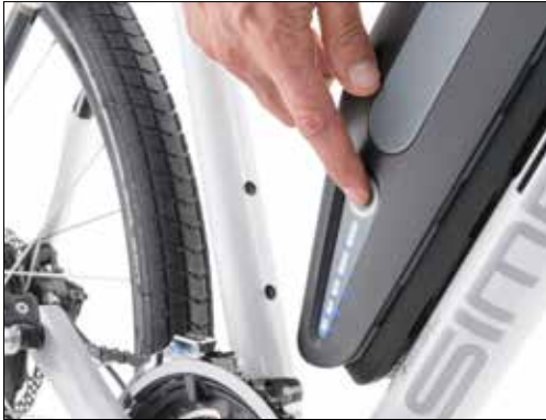
External battery: press the battery button. Battery button position may vary.
