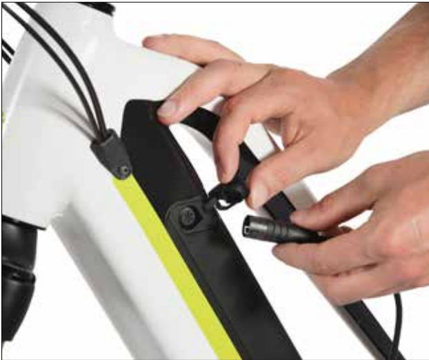
Battery charging, plugging in battery charger, UR-V7 battery
