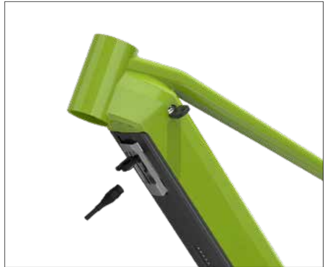
Battery charging, semi-integrated battery UR-V8
