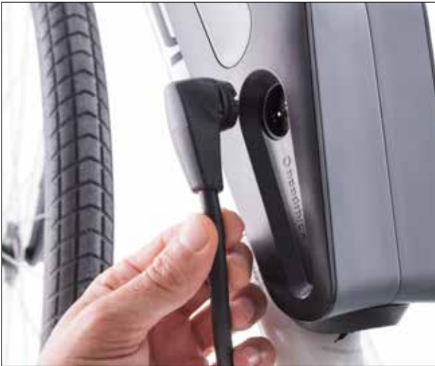
Battery charging, plugging in battery charger, UR-V2 battery
