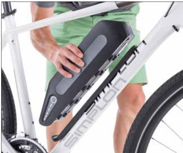
Inserting the external battery UR-V2
